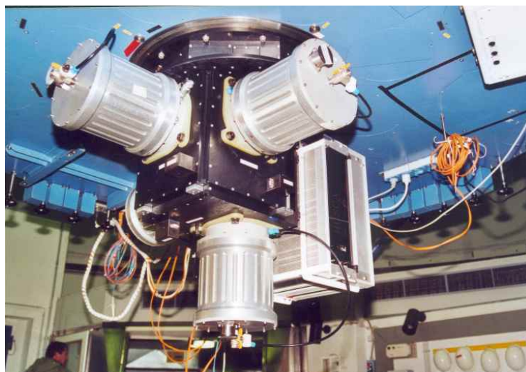
Figure 6.2: BUSCA with its four CCD systems mounted at the mirror cell of the 2.2m telescope. Copyright: CAHA
