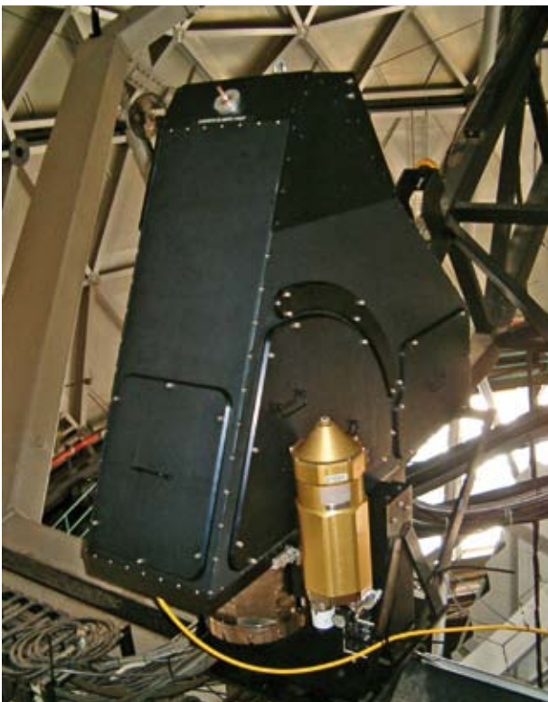
Fig. 5: VIRUS-P spectrograph mounted at the prime focus of the Hobby-Eberly Telescope.
