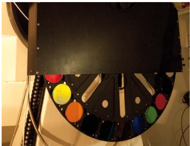
Fig. 3: The Wide-Field STELLA Imaging Photometer (WiFSIP) during installation.
