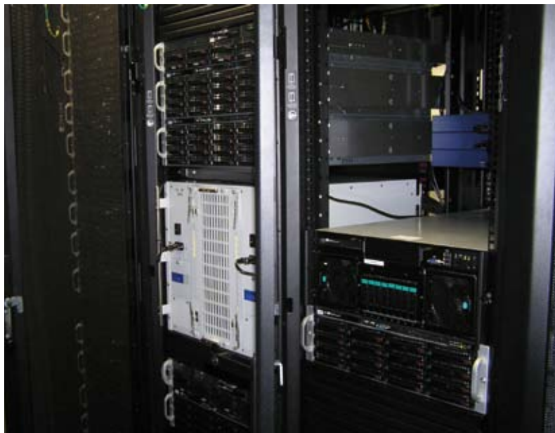
Fig. 2: Part of the GrayWulf cluster Almagest with Infiniband switch and main server erebos.aip.de for the CLUES project.
