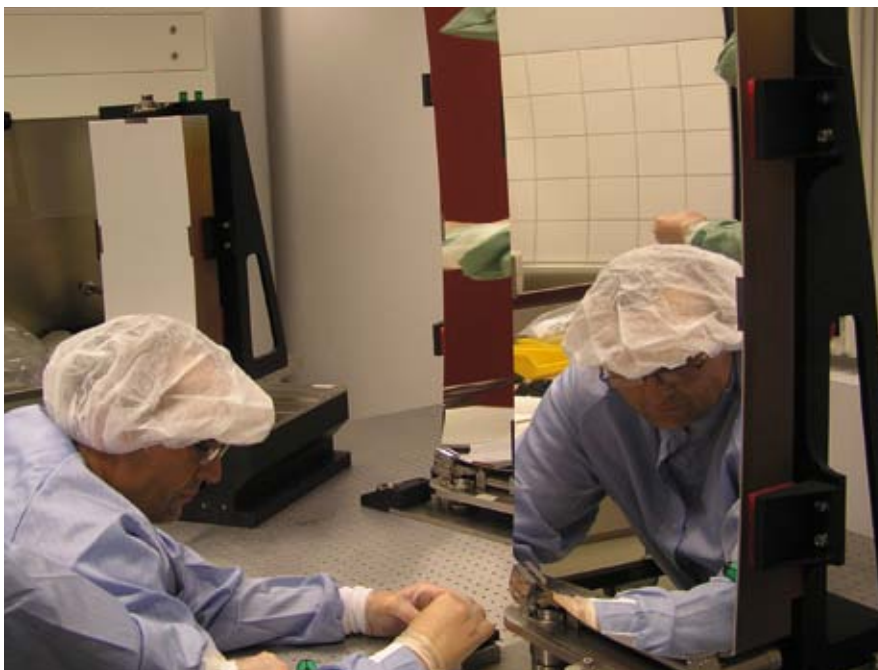
Collimators: Mounting the PEPSI mirrors in the AIP optical lab.
