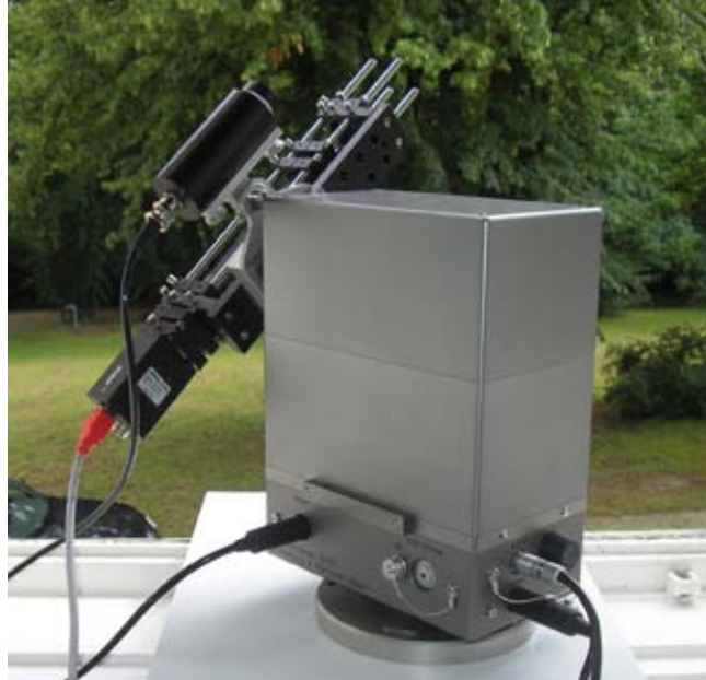
Prototype of the Solar Disk Integrated (SDI) telescope, pointed at the Sun over the Babelsberg campus.
