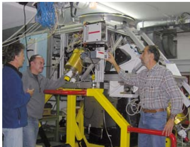
Fig. 8: Martin Roth, Thomas Fechner and Emil Popow (from left to right) install the new CCD detector at the PMAS instrument.
