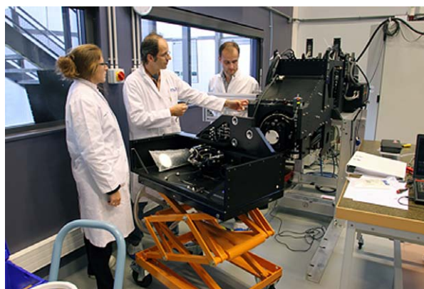
Fig. 1: Integration of the AIP-built MUSE calibration unit onto the fore-optics subsystem in Lyon.
