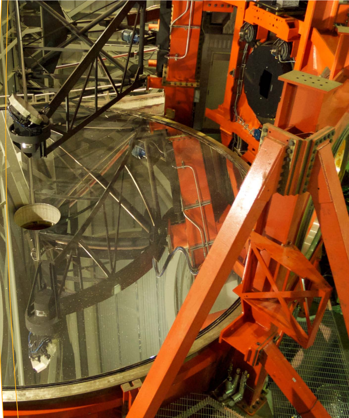
Left LBT primary and tertiary mirror. The location of the PEPSI Permanent Fibre Focus Units (PFU) is on the bracket at the right.
