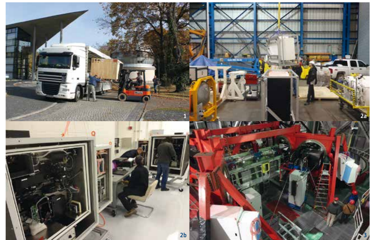
Fig. 4: The two PFUs for PEPSI on their way from AIP to the LBT: 1: AIP and LBT personnel working together on this delicate step. 2a+b: arrival on Mt. Graham, functionality tests in the pier, mounting on the telescope. 3: final home of the PFUs (white boxes) on the Nasmyth instrument platform in the bent Gregorian foci of the telescopes.
