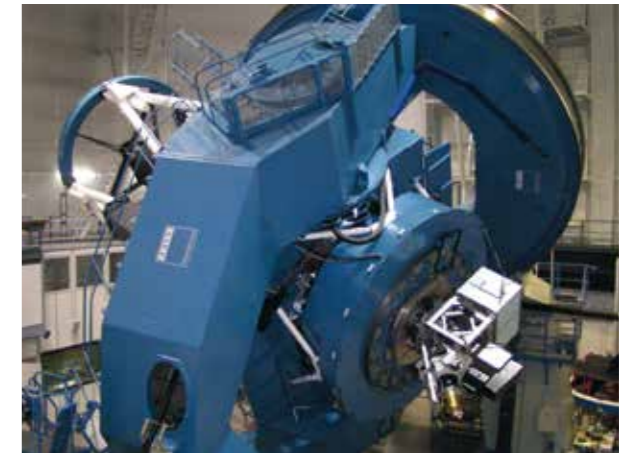
Fig. 5: The Potsdam Multi-Apertur Spektrophotometer (PMAS), mounted at the back of the Calar Alto 3.5m telescope.
