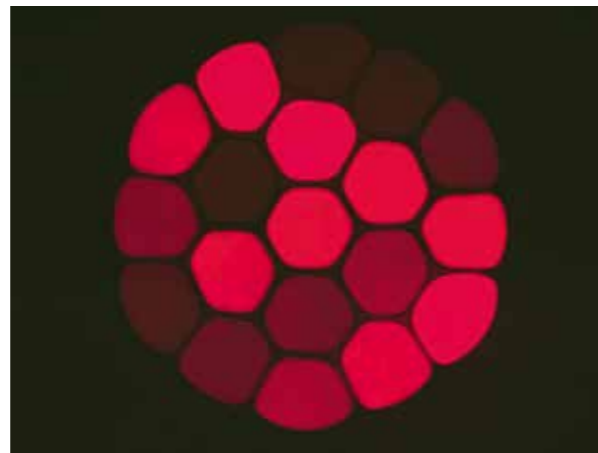
Fig. 8: Miniaturised and fused fibre bundles are investigated for suitability as deployable integral field units for multiplex 3D spectroscopy.
