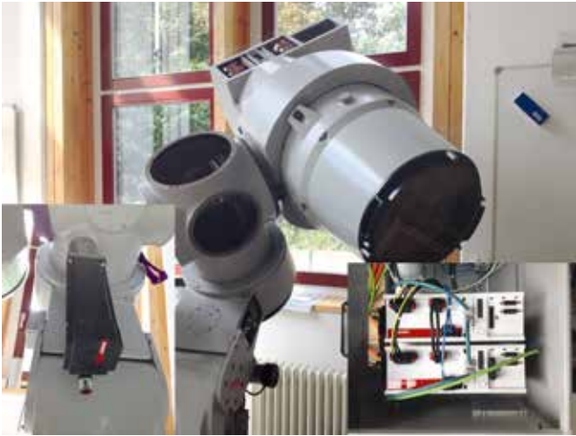
Fig. 3: Umbau von BMK10k: Ersetzen des alten Antriebs durch moderne Beckhoff-Servomotoren. BMK10k at refurbishment: replacement of the old drives with new servo motors from Beckhoff.
