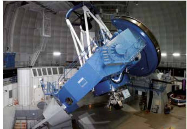
Fig. 8: Das Potsdam Multi-Aperture Spektrophotometer (PMAS) am Calar Alto 3,5-Meter-Teleskop. The Potsdam Multi-Aperture Spectrophotometer (PMAS) mounted below the 3.5m Calar Alto telescope. (Credit: Santos Pedraz, CAHA)
