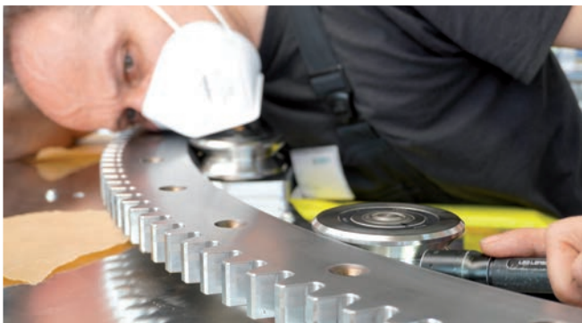
Arbeiten am 4MOST Cassegrain Cable Wrap (CaCW). Working on the 4MOST Cassegrain Cable Wrap (CaCW).
