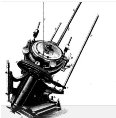
Fig. 16 Heliostat by Vogel and Lohse as part of the flagship of the observatory. Optics by Steinheil (Munich), mechanics by Repsold (Hamburg). With a device made by the same manufacturers in 1890, Schwarzschild attempted to measure the gravitational redshift of the nitrogen line 3883 \text{ \AA} on the roof of the Beamtenwohnhaus in 1913. Lohse (1889).
