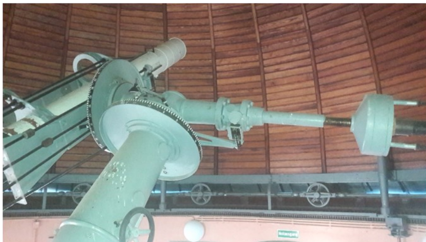
Fig. 41 Grotrian's coronagraph (guide tube), 13 cm refractor with 190 cm focal length, originally set up in the Miethe dome in 1952, now in the east dome of the main building (now the Michelson House of the Potsdam Institute for Climate Impact Research). Lens still available (information J. Rendtel).
