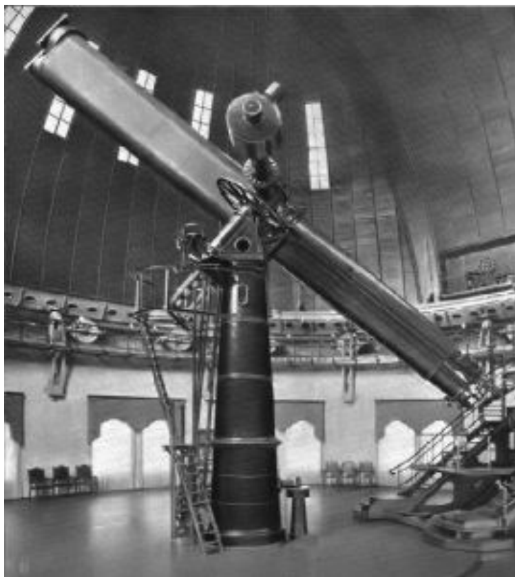
Fig. 24 Great refractor from 1899, dome 21 m, astrograph 80 cm, visual guide tube 50 cm, focal lengths slightly more than 12 m, mechanics by Repsold. electric (gas-powered dynamo) by Siemens & Halske. Unlike other designs, the floor is rigid, but the observation chair is rigidly attached to the dome. "The optical 50-cm-lens proved to be quite excellent during the examination with the exclusion of a narrow edge zone." 137 The astrograph was the problem: Steinheil had tried to save the 300 kg lens in Potsdam in May 1900 and in Munich in January 1904 without success. 138
